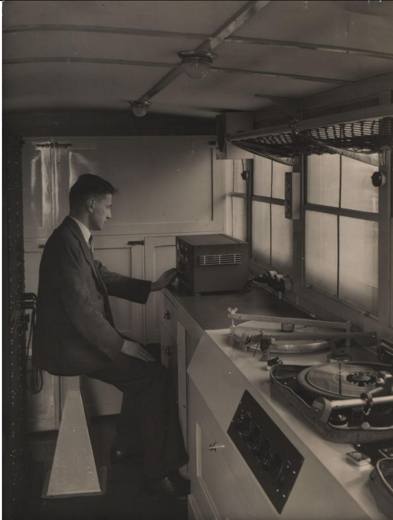
Interior of the Mobile Broadcasting Unit truck in Egypt, with Noel Palmer and disc cutting equipment. (RNZ photographic collection, Ngā Taonga Sound & Vision.)
